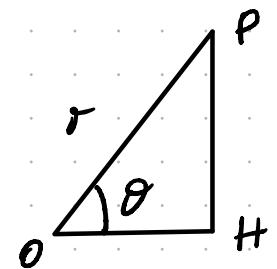
$$\overline{PH} = \overline{OP} \sin \theta \rightarrow \sin \theta = \frac{\overline{PH}}{r}$$
